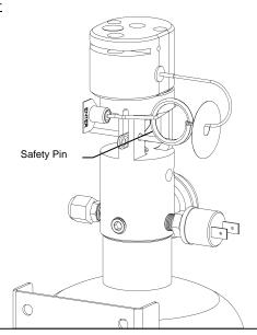
Extinguisher should be securely mounted and Cable should be routed. Be sure the Safety Pin is in place.
