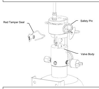
With T-Handle previously secured, remove Red Tamper Seal from Extinguisher to remove Safety Pin and store in provided hole.
