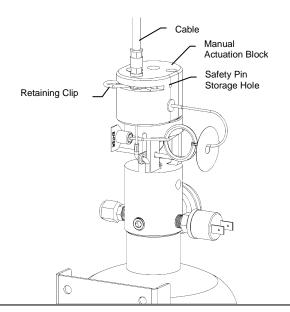
Secure Cable into Manual Actuation Block with Retaining Clip.
