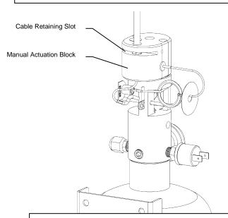
Insert extinguisher end of Cable through hole in Manual Actuation Block past retaining slot on Cable.
