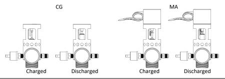
Disconnection and Inspection of Manual Discharge Cable
