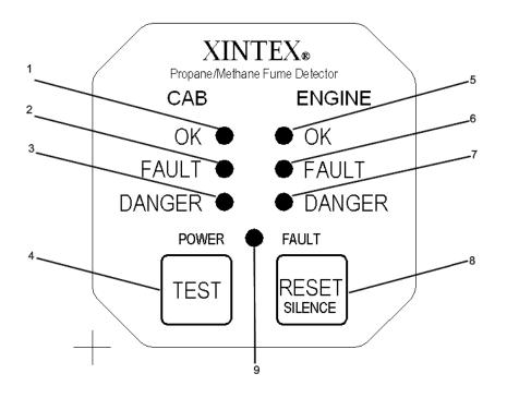
**CAUTION**: NO POWER ON/OFF SWITCH IS PROVIDED FOR THIS UNIT. TO FUNCTION AS INTENDED, THE S2B-M-X2 MUST BE CONNECTED TO A CORRECT POWER SOURCE, AND FOR MAXIMUM EFFECTIVENESS, BE POWERED AT ALL TIMES A DANGER MAY BE PRESENT. IF POWER IS ON AND LEFT UNATTENDED FOR AN EXTENDED PERIOD OF TIME, BATTERY POWER MAY BE DIMINISHED.
