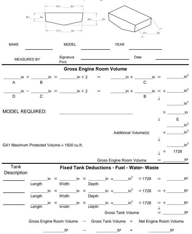
USCG & ABYC ALLOWS DEDUCTIONS FOR FIXED TANKS BY BOAT MANUFACTURERS ONLY. NOTE: ENGINE VOLUME CANNOT BE DEDUCTED
