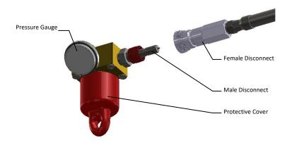
Connect Hose to Extinguisher. There should be an audible click. The male connector will be under pressure, which will require more force to make the connection.
