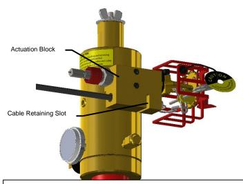
Insert extinguisher end of Cable through hole in Actuator Block past retaining slot on Cable.
