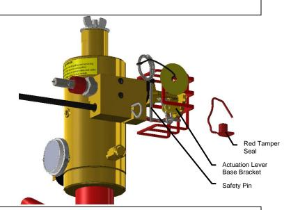
With T-Handle previously secured, remove Red Tamper Seal from Extinguisher to remove Safety Pin and store in provided location.
