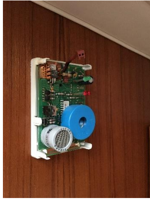
Squeeze cover and remove and unplug connector
