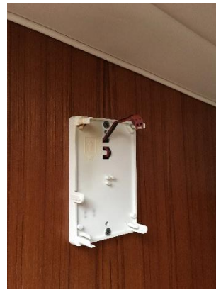
Bend bottom corner prongs outward and remove circuit board Remove two screws and bracket
