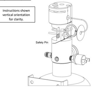
Extinguisher should be securely mounted and Cable should be routed. Be sure the Safety Pin is in place.
