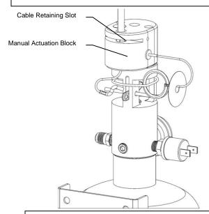
Insert extinguisher end of Cable through hole in Manual Actuation Block past retaining slot on Cable.
