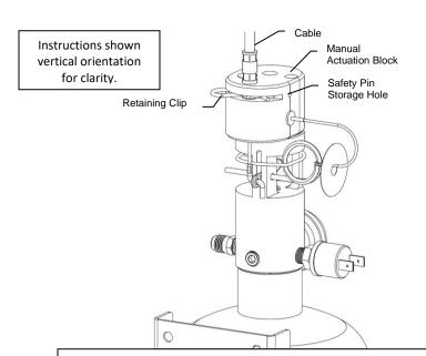
Secure Cable into Manual Actuation Block with Retaining Clip.
