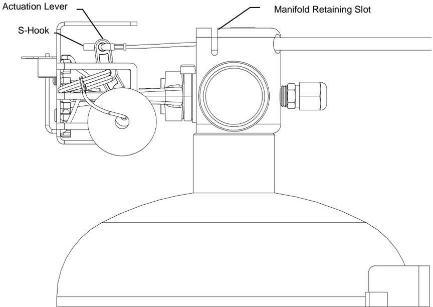
Align retaining slot of Cable with retaining slot of Manifold.
