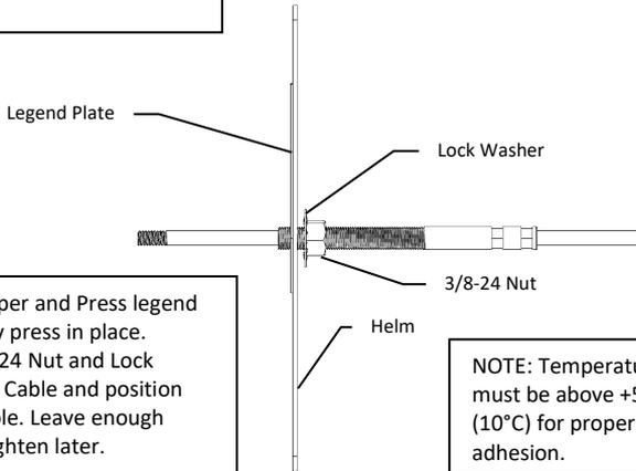
Peel off paper and Press legend plate firmly press in place. Install 3/8-24 Nut and Lock Washer on Cable and position through hole. Leave enough space to tighten later.
