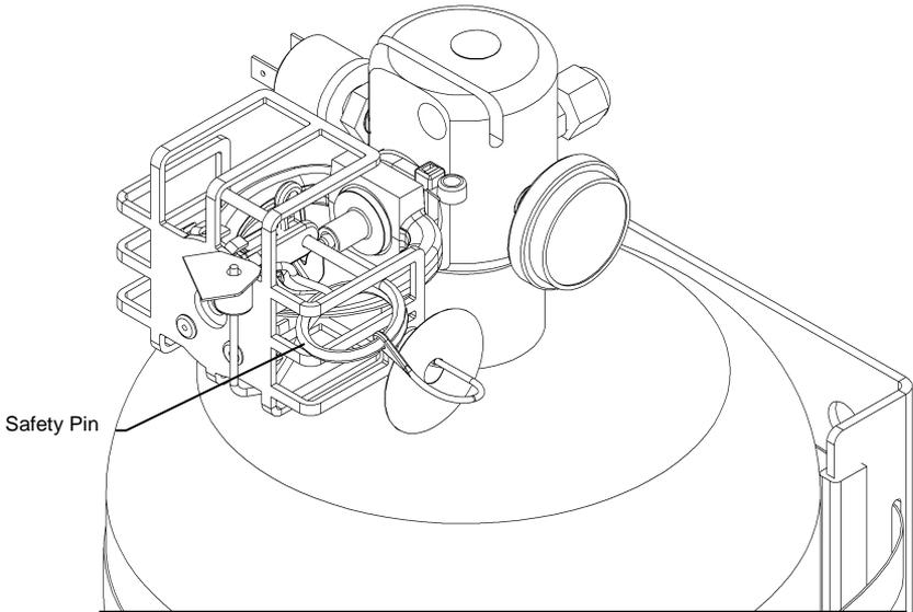
Extinguisher should be securely mounted and Cable should be routed.
