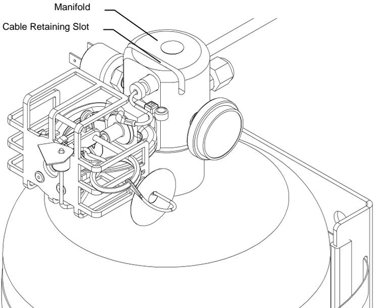
Insert extinguisher end of Cable through hole in Manifold past
