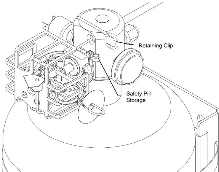
Secure Cable to Manifold with Retaining Clip.
