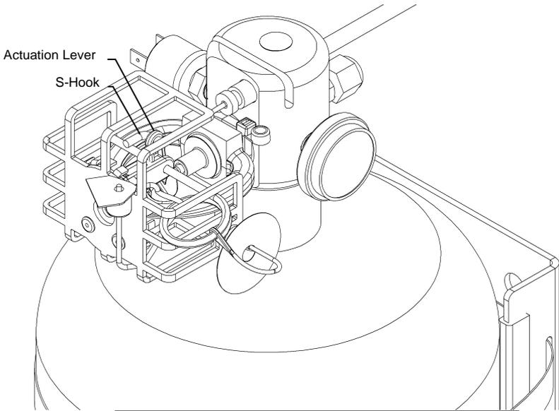
Insert S-Hook into hole at the top of Actuation Lever.
