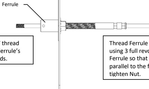
Note: Do NOT thread further than Ferrule's internal threads.
