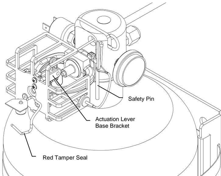
With T-Handle previously secured, remove Red Tamper Seal from Extinguisher to remove Safety Pin and store in provided location. Cable system is now operational.
