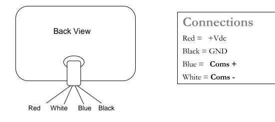
Power and Comms Wiring Connections:
