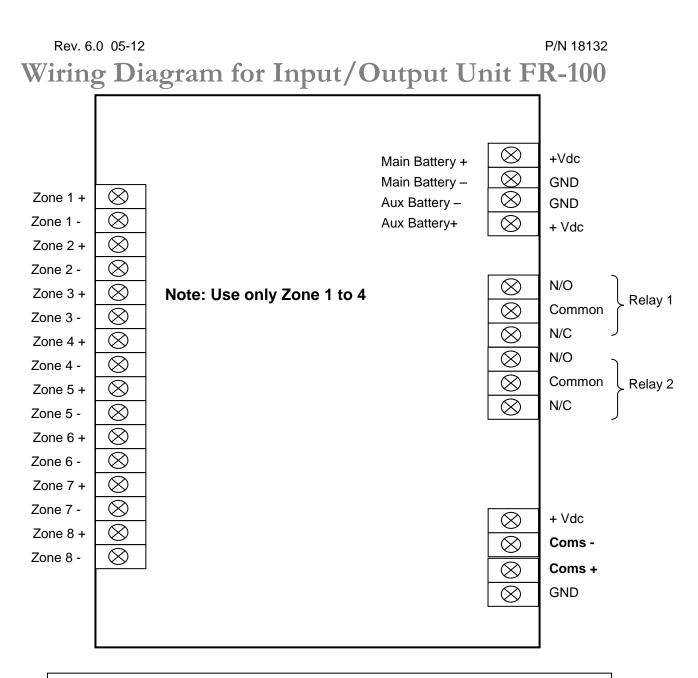
Note: If you require the Aux Battery to be charged by the Main Battery supply then fit D1charging diode (IN 5404) as per below. The stripped band on the diode should be connected to the Aux Battery + terminal.
