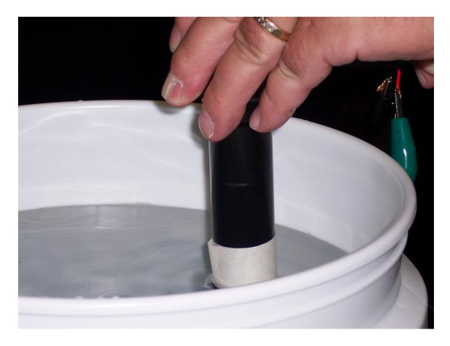
Step 12: Submerge the sender to the level at which you want the display to read "full" (factory setting is 2" from the top of the sender)
