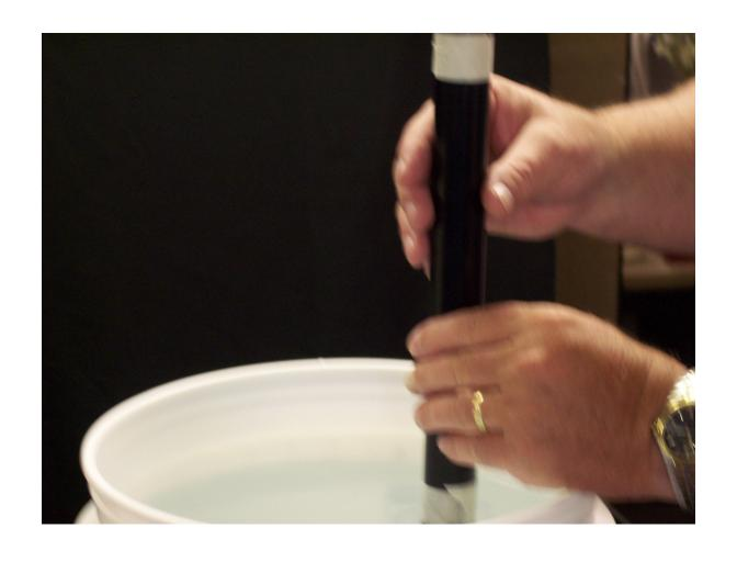
Step 10: Submerge the sender to the level at which you want the display to read "empty"
