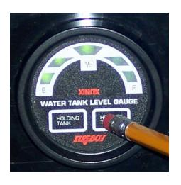
Step 14: Snip the exposed green and white wires back to avoid accidental entry into calibration mode. Empty, half and full level displays shown above.\*
