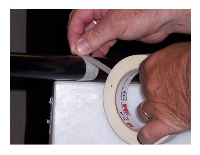
Step 3:Score the surface of your sender to mark the cutting line (or mark with masking tape as shown above)
