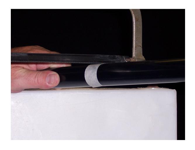
Step 4: Carefully cut the sender using a fine-tooth, hand held saw (Secure tightly to avoid damaging vibrations)
