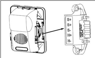
The access holes are provided in the back of the terminal block to allow the voltage to be measured directly without removing the device. Typically this would be done at the end of the line to confirm design criteria. Most measurements will be taken using the S+ and S- locations although access is provided to other locations. NOTE: Care should be taken to not short the test probes.
